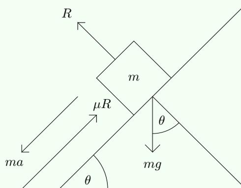
Hence, the component of  $mg$  perpendicular to the plane is  $mg \cos(\theta)$ .
