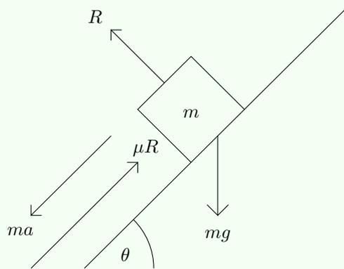
We resolve forces parallel to the plane and perpendicular to the plane. This is because  $ma$  acts parallel to the plane so we want to resolve forces in the same direction as  $ma$  in order to make the problem as simple as possible.
